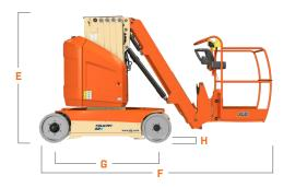
Platform Width 41.3-in / 1.05-m A. Platform Length 27.5-in / 0.70-m В. Machine Width 3-ft 9-in / 1.20-m 5.9-in / 15-cm Tailswing Machine Height 6-ft 5-in / 1.99-m Ε. Machine Length 12-ft / 3.65-m (Drop Bar) Wheelbase 5-ft 3-in / 1.60-m H. Ground Clearance 3.9-in / 10-cm
